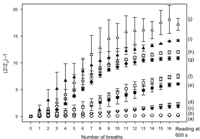
**Fig. 6.** Relationship between ratiometric impedance response and number of cumulative simulated breaths of 4 s duration. Ammonia concentrations were: (a)  $40 \pm 2$ ; (b)  $121 \pm 15$ ; (c)  $245 \pm 8$ ; (d)  $392 \pm 6$ ; (e)  $755 \pm 7$ ; (f)  $984 \pm 21$ ; (g)  $1368 \pm 11$ ; (h)  $1576 \pm 7$ ; (i)  $1919 \pm 20$  and; (j)  $2175 \pm 26$  ppbv.
