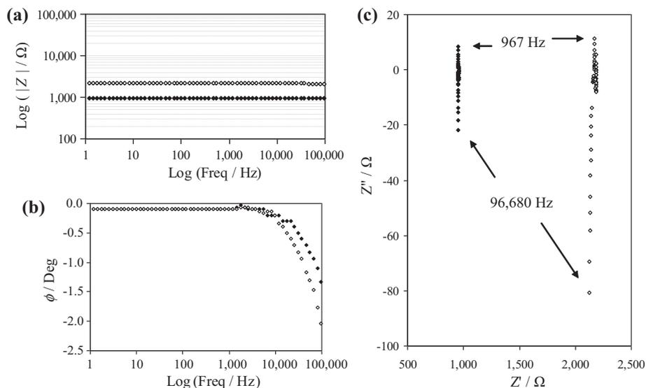
**Fig. 2.** Impedance and phase behaviour of polyaniline nanoparticle-modified electrodes before (filled diamonds) and after (empty diamonds) exposure to 25 ppmv ammonia. Results over the frequency range of 1 Hz to 100 kHz are indicated by (a) Bode, (b) phase and (c) Nyquist plots.
