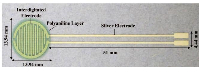
Fig. 1. Design of the interdigitated polyaniline nanoparticle modified electrode. Screen printed silver interdigitated electrodes were covered with multiple layers of an inkjet printed polyaniline nanoparticle dispersion forming a green film.
