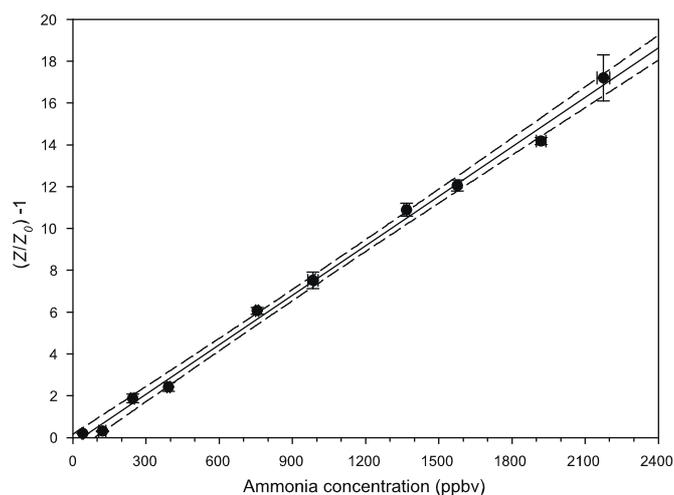
**Fig. 8.** Relationship between ammonia concentration and ratiometric impedance response after 16 simulated breath samples measured at 600 s ( $R^2 = 0.9963$ ). A slope and intercept of  $0.0079 \text{ ppbv}^{-1}$  and  $-0.2852$  were determined. 95% confidence interval (dashed line).
