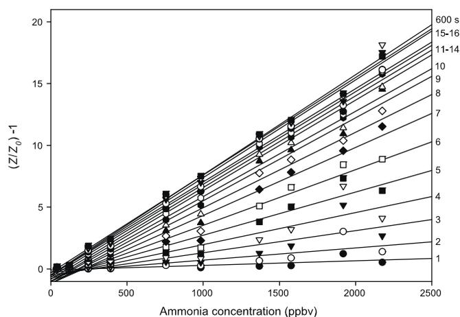
**Fig. 7.** Relationship between ratiometric impedance response and ammonia concentration with respect to the number of cumulative breaths (1–16) sampled. The value of 600 s indicates a final measurement at this time.
