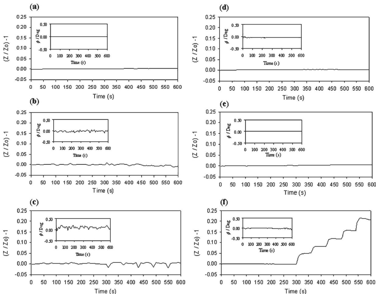
**Fig. 3.** Ratiometric impedance  $[(Z/Z_0)-1]$  and phase ( $\phi$ ) (inset) responses of the polyaniline nanoparticle-modified electrodes to potential interferent gases in human breath: (a) 99% (v/v) carbon dioxide, (b) 99% (v/v) nitrogen, (c) 99% (v/v) oxygen, (d) 25 ppmv hydrogen sulfide, (e) 25 ppmv nitric oxide, (f) 25 ppmv ammonia ( $n = 3$ ).
