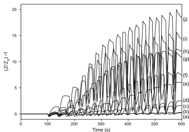
**Fig. 5.** Ratiometric impedance response  $[(Z/Z_0) - 1]$  profile of simulated breath samples of 4 s duration on polyaniline nanoparticle-modified electrodes measured at 962 Hz. The ammonia concentrations were: (a)  $40 \pm 2$ ; (b)  $121 \pm 15$ ; (c)  $245 \pm 8$ ; (d)  $392 \pm 6$ ; (e)  $755 \pm 7$ ; (f)  $984 \pm 21$ ; (g)  $1368 \pm 11$ ; (h)  $1576 \pm 7$ ; (i)  $1919 \pm 20$ ; and (j)  $2175 \pm 26$  ppbv.
