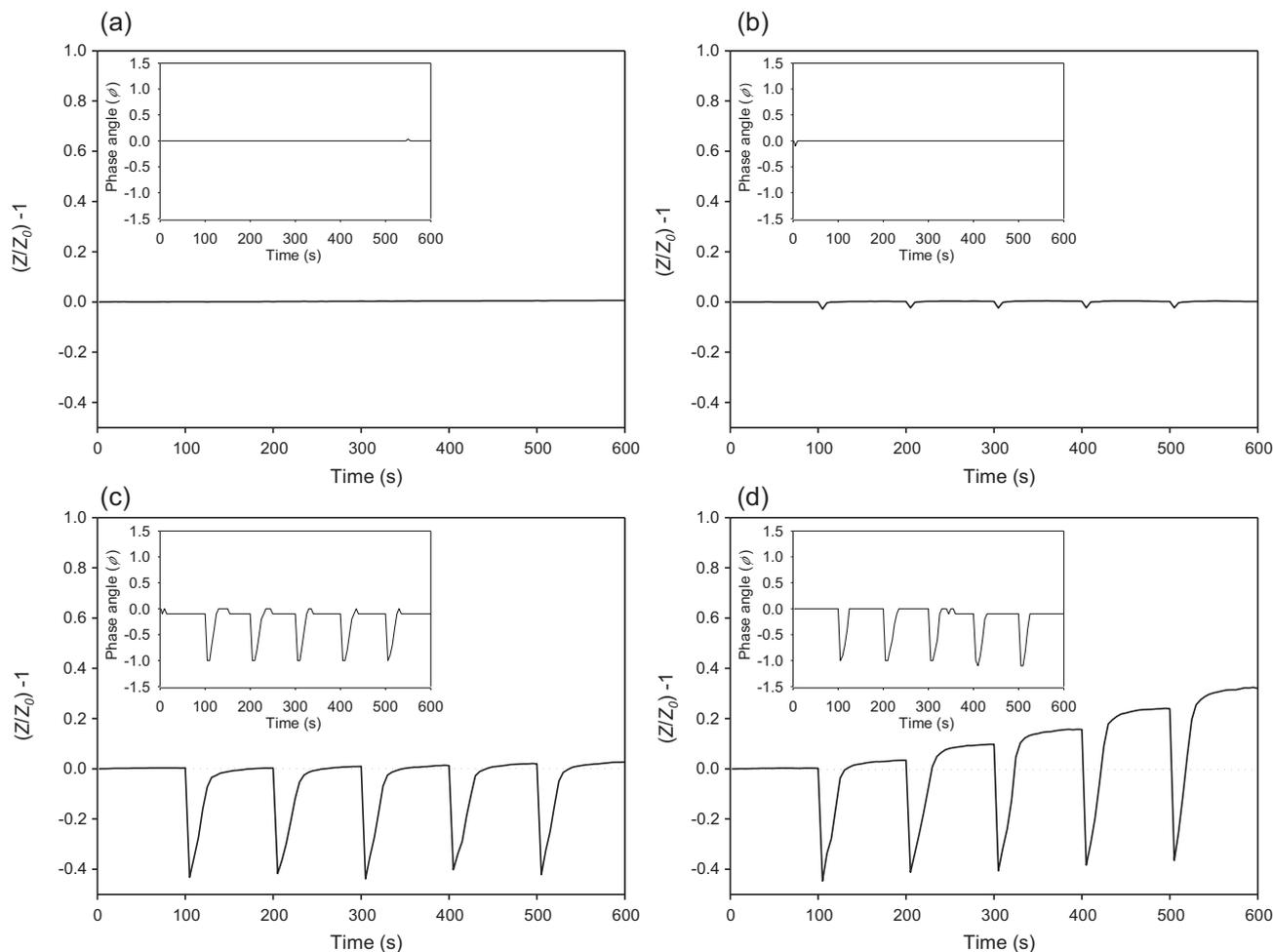
**Fig. 4.** Polyaniline nanoparticle-modified electrode ratiometric impedance responses  $[(Z/Z_0) - 1]$ , and phase angle ( $\phi$ ) (inset) to (a) room temperature atmospheric air,  $21 \pm 1^\circ\text{C}$ , (b) warmed atmospheric air ( $37 \pm 1^\circ\text{C}$ ), (c) warmed humidified atmospheric air ( $37 \pm 1^\circ\text{C}$ ,  $\geq 90\%$  RH) and (d) warmed humidified air with ammonia ( $37 \pm 1^\circ\text{C}$ ,  $\geq 90\%$  RH,  $245 \pm 8$  ppbv).
